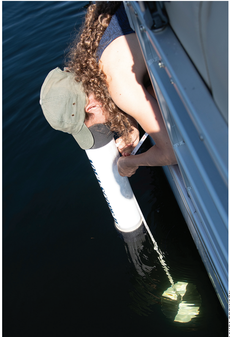
Peering through aquascope toward Secchi disk to determine water quality
