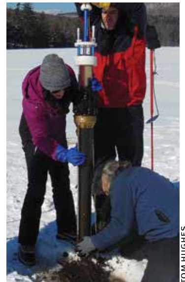
Taking a core sediment sample at Horseshoe Pond.
